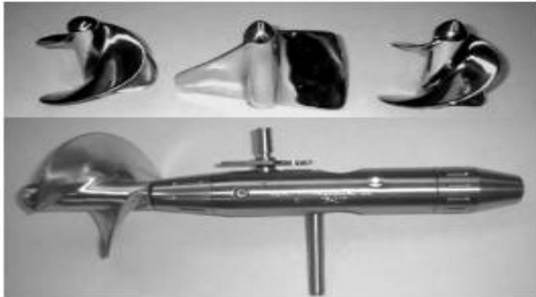
Рис. 11. Universal Current Meter – Model 6500 (Ricky Hydrological Company, США) (по [12; 19])
