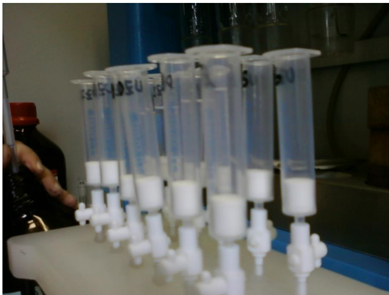
2.2-rasm. "Strata Solid Phase Extraction" ichiga sorbent solingan kolonkalar.
