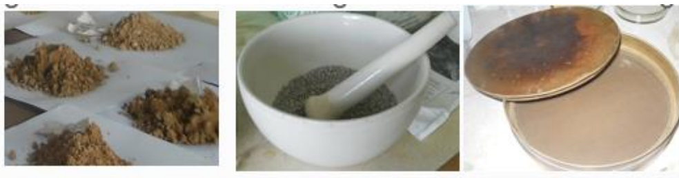
2.4-rasm. Tuproq namunasini quritish va gomogenlashtirish
