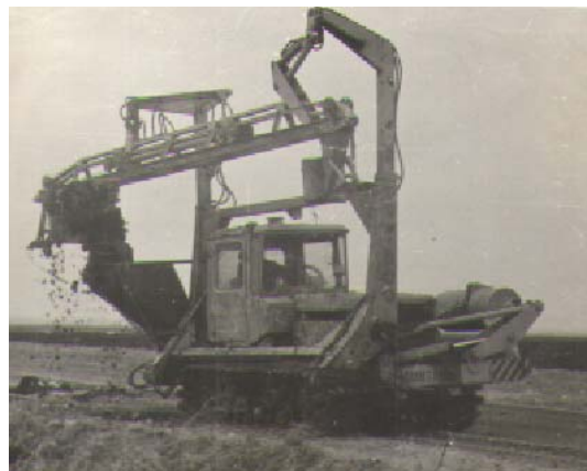
Figure 2. Discharge of sediment from the bucket to the ground receiving device-slip.
