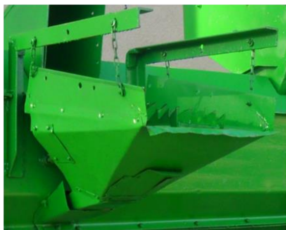
Figure 2. Experimental sample of sieve of the corn-thresher machine
