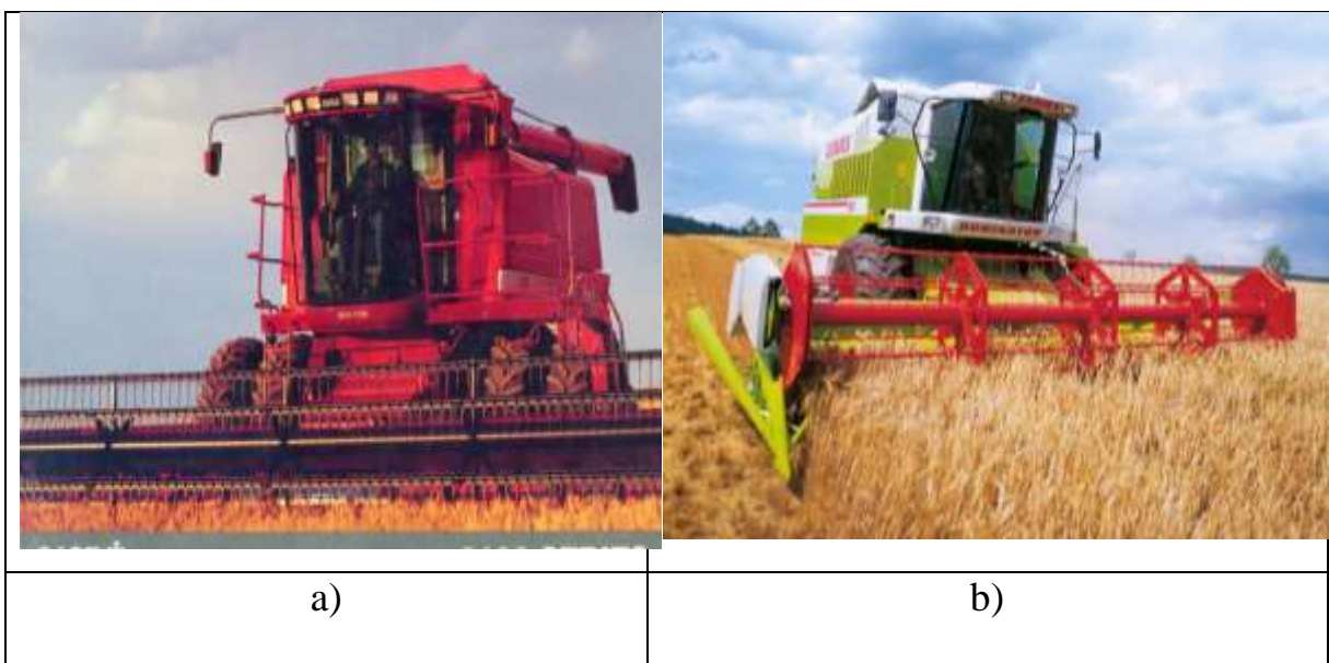
10.3-rasm. “Keys–2166” rusumli aksial-rotorli (a) va “Dominator - 130”rusumli barabanli (b) g’alla kombaynlari
