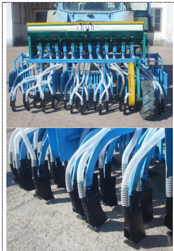
Figure 3. Seeder for cotton rows and special coulters
