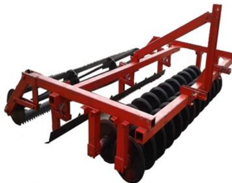
Figure 1. The combined machine used in the processing of new plowed field.
