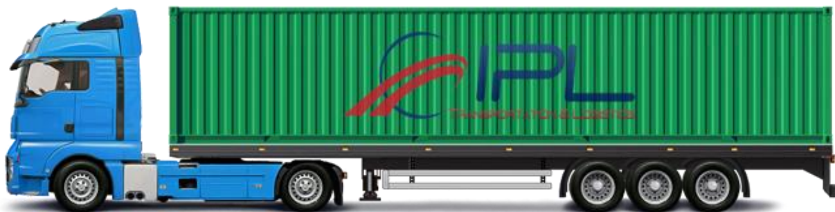
24-rasm. 40 futli konteynerga ega bo'lgan 20 tonnalik fura
