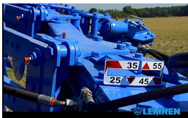
31-rasm. Lemken firmasi plugining qamrash kengligini o‘zgartirish innovatsion qurilmasi
