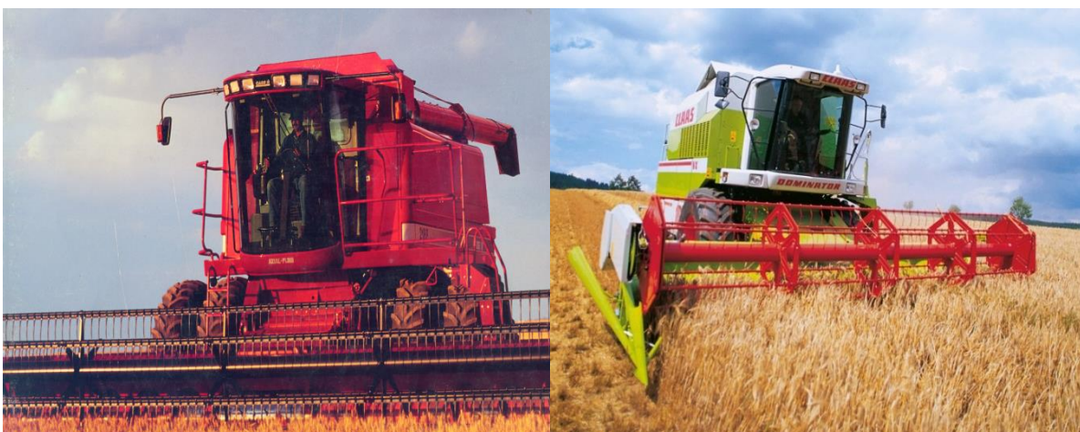
58-rasm. "Keys-2166" rusumli aksial-rotorli (a) va "Dominator - 130" rusumli barabanli (b) g'alla kombaynlari
