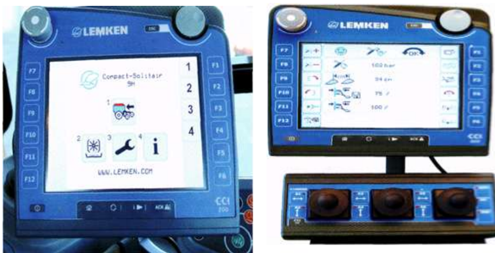
25-rasm. Belgilar va piktogramma qurilmasi (a) va plugni boshqarish uchun djoystli SSIISOBUS terminali (v)
