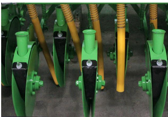
98-rasm. Don ekish seyalkasining mexanizmlari
