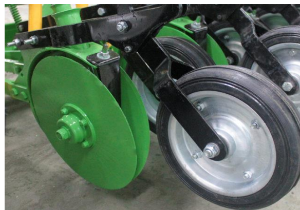
98-rasm. Don ekish seyalkasining mexanizmlari
