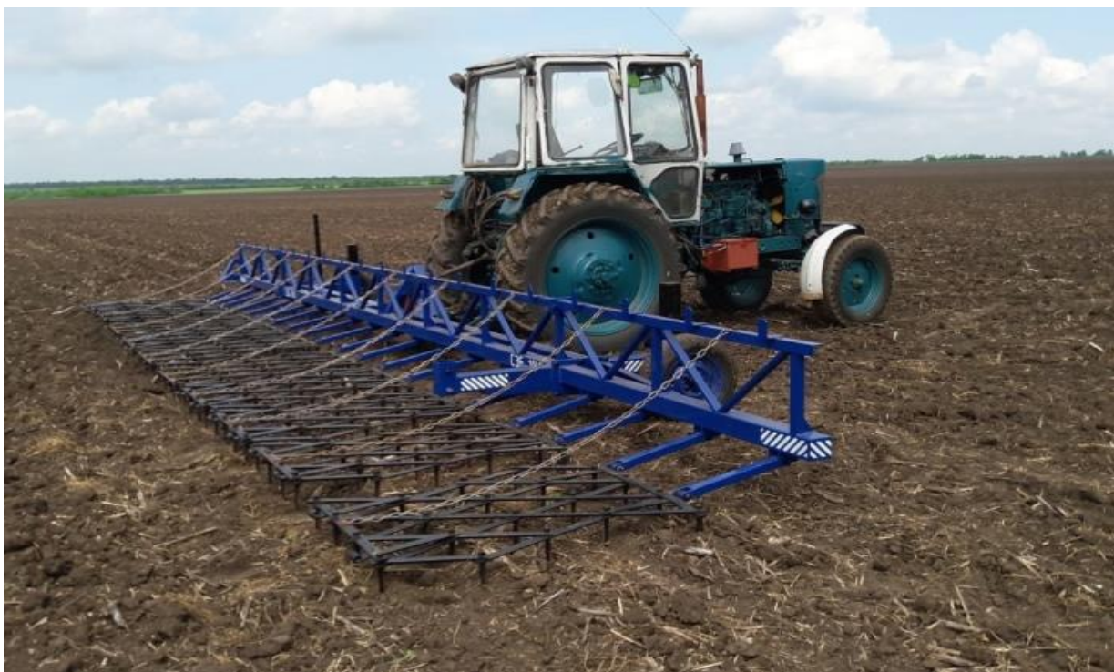
50-rasm. G'ildirakli traktor bilan tuzilgan boronalash agregatining ish jarayini
