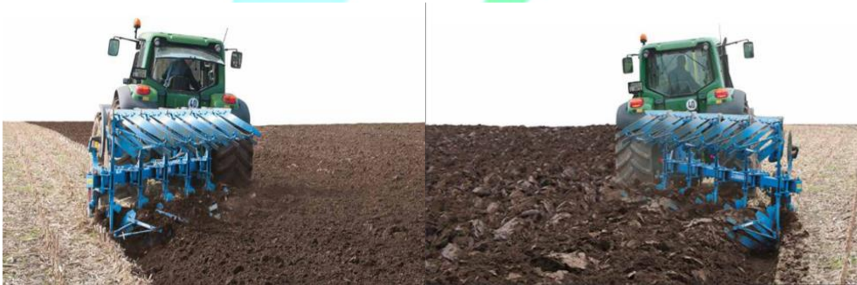
2-rasm. Ag'darma plugli mashina-traktor agregatining dala matdoni bo'yich borib-kelishdagi shudgorlash jarayoni
