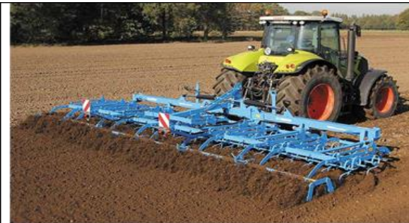
9-rasm. Dalaga yuza ishlov beradigan mashina-traktor agregati
