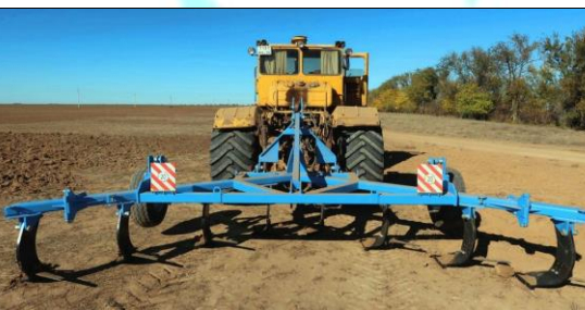
8-rasm. Yerni chuqur yumshatadigan mashina-traktor agregati
