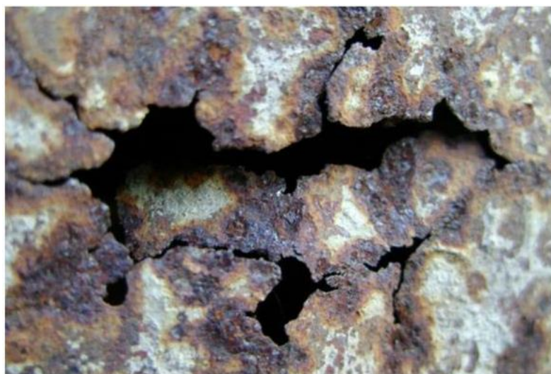
15-rasm. Korroziyadan yorilish (emirilish)
