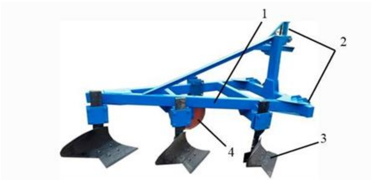
1-rama, 2-osish qurilmasi, 3-korpus, 4-tayanch g'ildirak 20-rasm. PN-3-30 uch korpusli osma plug
