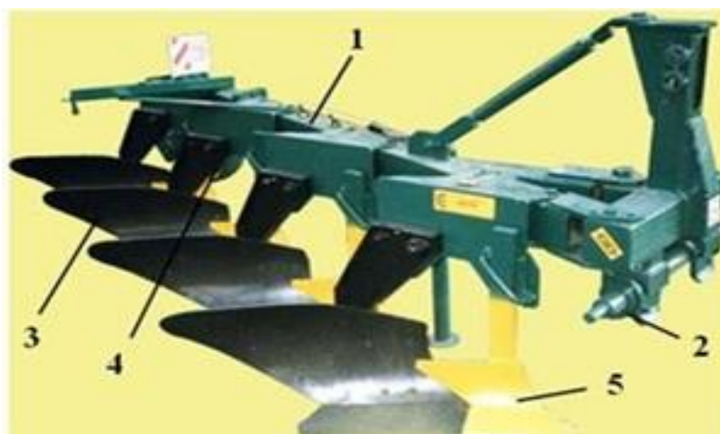
1-rama, 2-osish qurilmasi, 3-korpus, 4-tayanch g'ildirak, 5-chimqirqar 21-rasm. PNR (3+1)x45 osma plug
