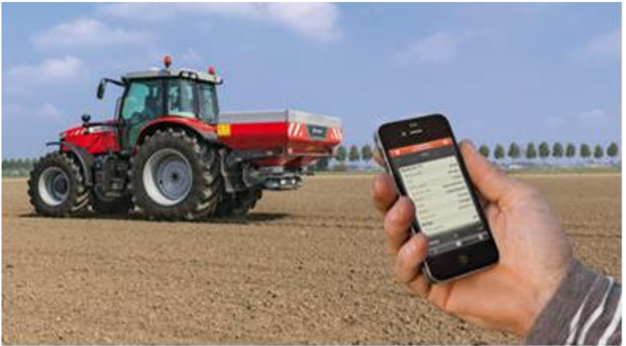
9-rasm. Tarqoq (sochish) usulda mineral o‘g‘it sohadigan yuqori unumli mashina
