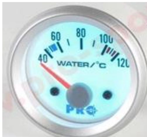
29-rasm. Sovutish suyuqligining haroratini o'lchagich
