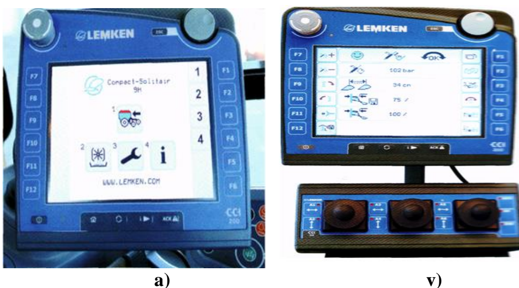
47-rasm. Belgilar va piktogramma (a) qurilmasi va plugni boshqarish uchun djoystli SSI ISOBUS (v) terminali
