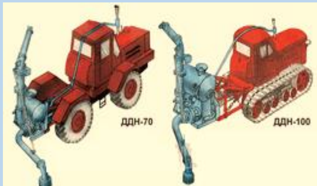
52-rasm. a-DDA-100M; b-DDN-70; v-DDN-100 yomg‘irlatib sug‘orish agregatlari
