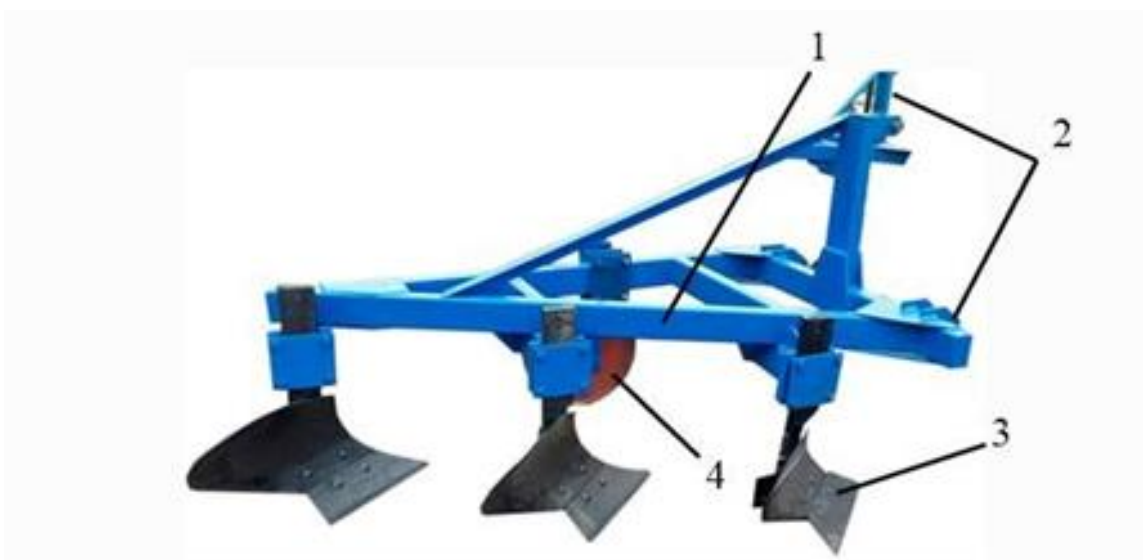
1-rama, 2-osish qurilmasi, 3-korpus, 4-tayanch g'ildirak 18-rasm. PN-3-30 uch korpusli osma plug
