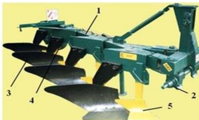
1-rama, 2-osish qurilmasi, 3-korpus, 4-tayanch g'ildirak, 5-chimqirqar 19-rasm. PNR (3+1)x45 osma plug
