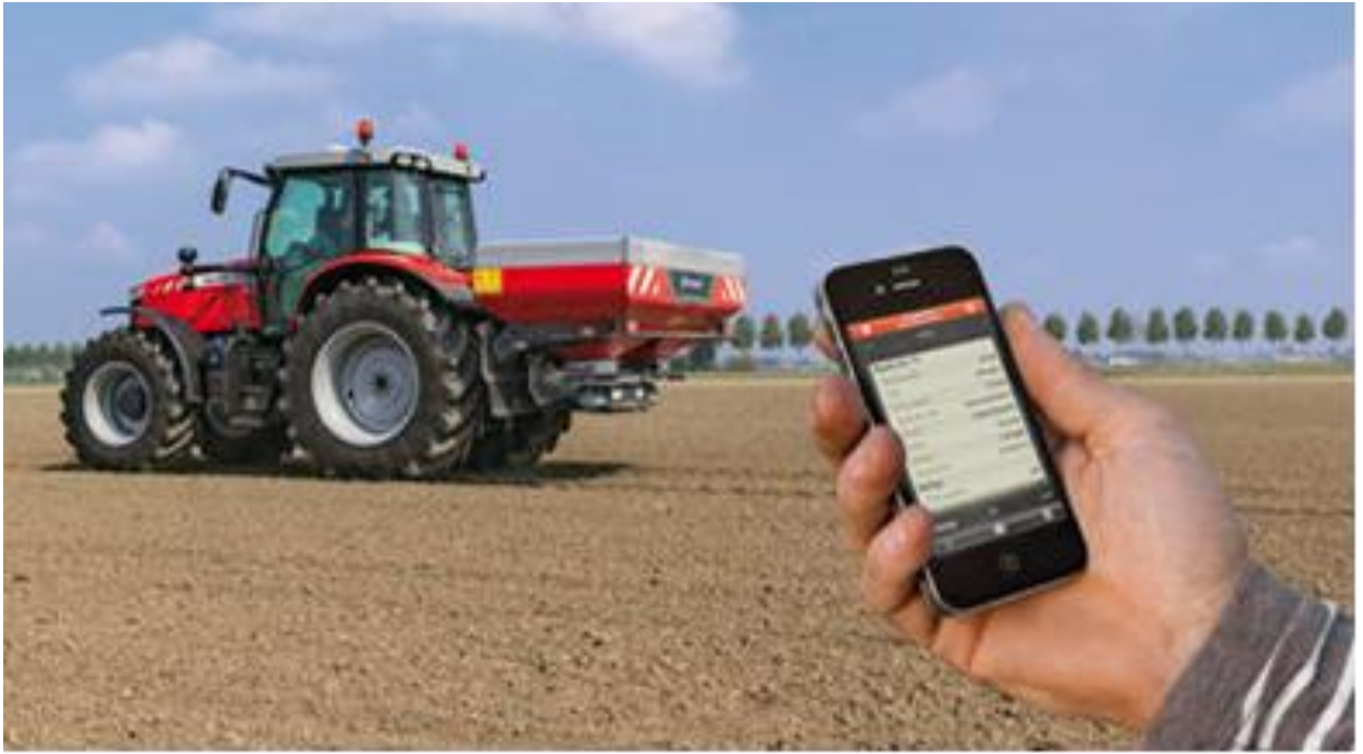
9-rasm. Tarqoq (sochish) usulda mineral o'g'it sochadigan yuqori unumli mashina
