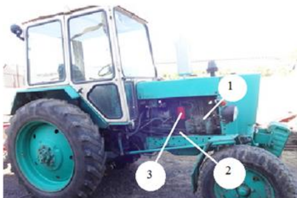
Figure 9. A view of the fuel-liquid heating device installed on the tractor. 1-high pressure pump; 2nd coarse cleaning filter; 3-temperature stimulator.
