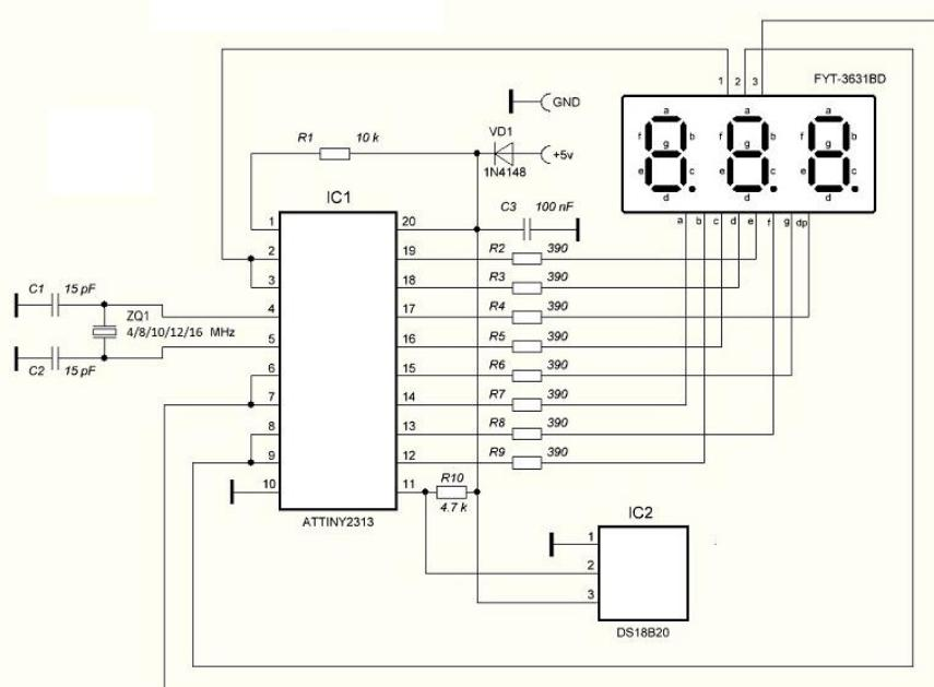
1 – rasm. Termogigometrning elektron chizmasi
