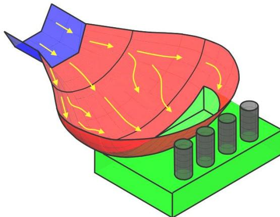
**Fig: 5. Computer model of the advance chamber**
