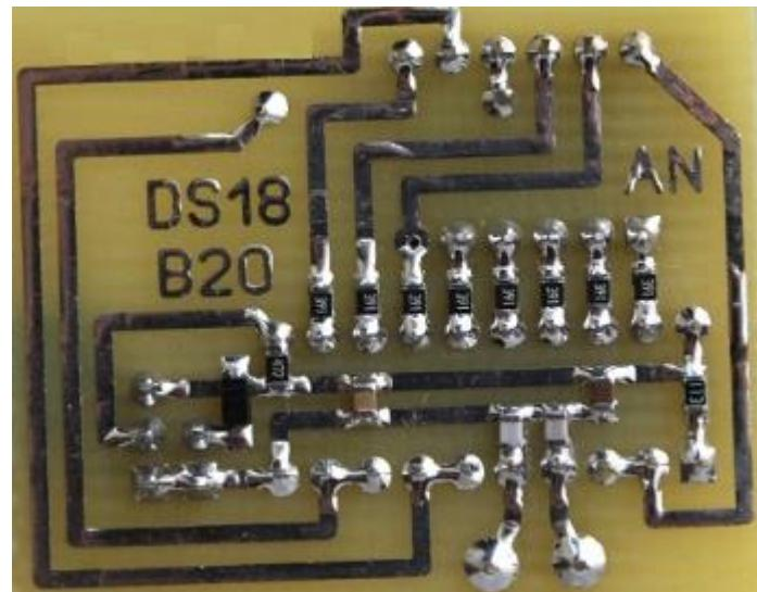
2 – rasm. Elektron chizmaga asoslanib yig'ilgan Termogigrometr.
