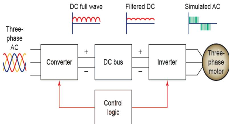
Fig. 1. Block diagram of the VFD Control Systems
