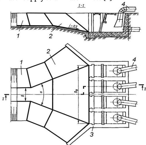
Fig. 1. Scheme of the water intake structure.
