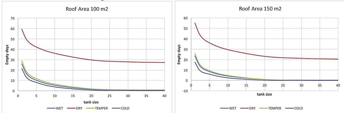
Fig 3. Combinations of 100 m<sup>2</sup> and 150 m<sup>2</sup> roof and tank sizes
