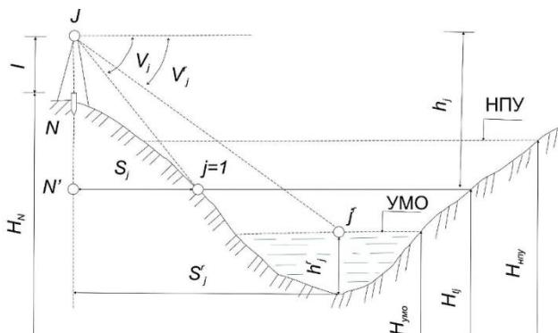
Putting on the tablet, according to the coordinates, the points of the shooting justification and laying off the distances  $S_j$  from them according to formula (1) for known directions  $\beta_j$ , find the position of each point  $j$ .
