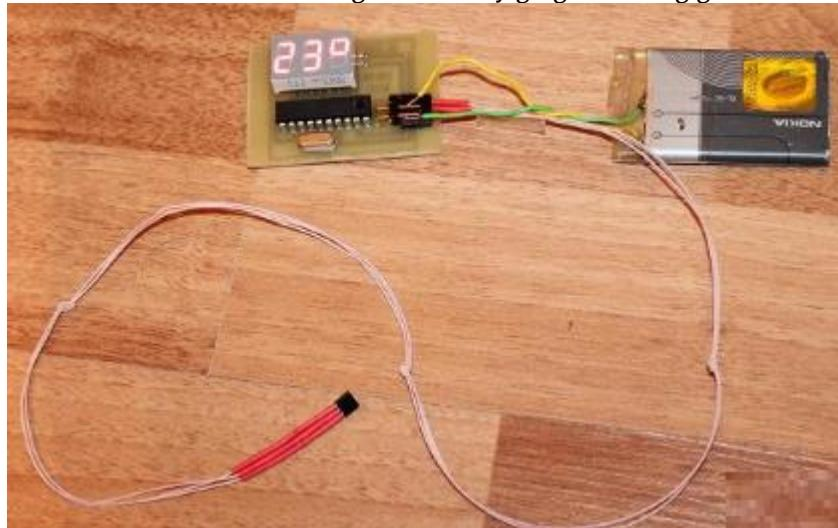
3 – rasm. Termogigrometrning tayyor holati.
