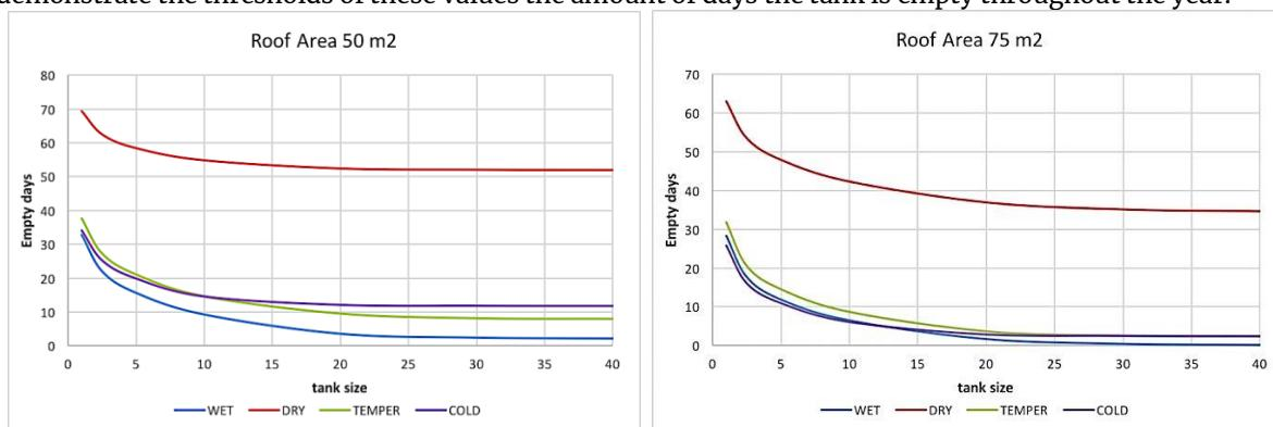
Fig 2. Combinations of 50 m<sup>2</sup> and 75 m<sup>2</sup> roof and tank sizes
