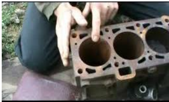
45-rasm. Tsilindr blokini organoleptik usul yordamida tekshirish
