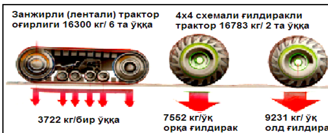
4.5-rasm. Traktor yurish qismining tuproqning chuqur zichlanishiga ta'siri
