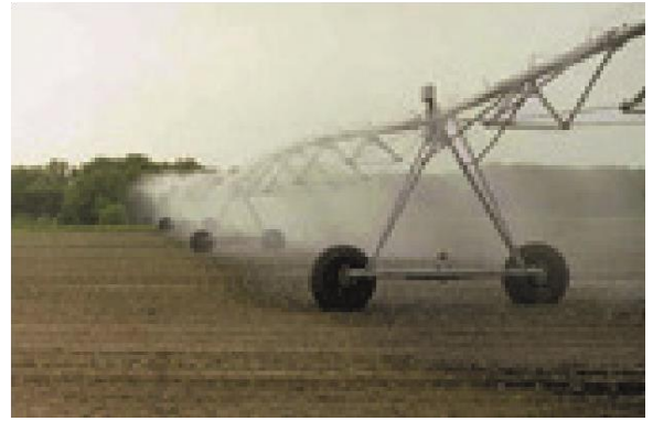
2.4.8-rasm. Yomg'irlatib sug'orish tizimining ishlash jarayoni
