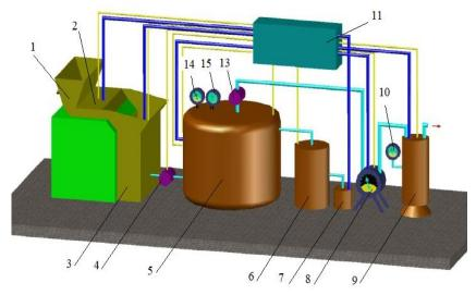
Fig.2. Scheme of an experimental plant for anaerobic processing of organic waste from birds 1-container for receiving organic waste; 2-boot device; 3-biomass grinder; 4- pump; 5-bioreactor; 6-container for biofertilizer; 7-separator; 8-gas generator; 9-gas filter; 10- gas meter; 11-panel rarefaction and mixing; 12-chopper; 13-vacuum pump; 14-management of the rarefaction mode; 15-thermometer.
