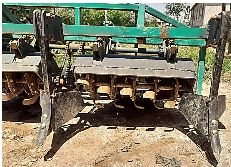
Figure 2. Milling drum (front view).
