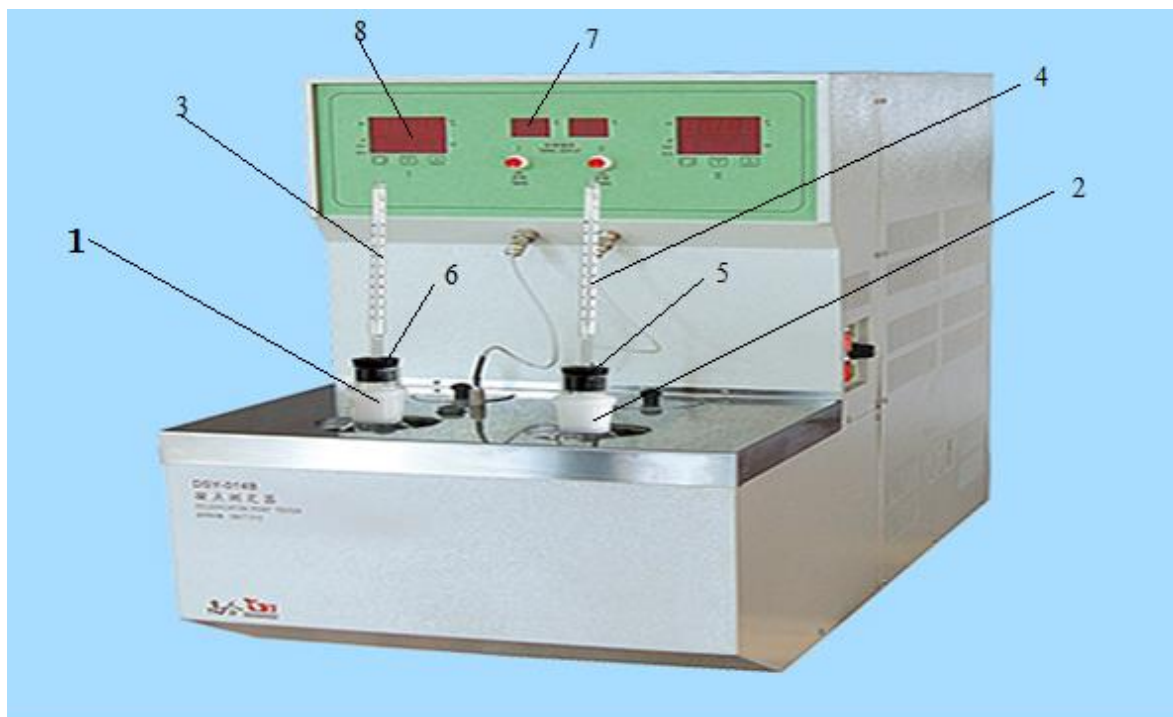
11-rasm. Neft mahsulotlarini hiralashish va qotish haroratini aniqlash. 1,2 - probirka; 3,4- termometr; 5,6- mufta, 7- vaqt hisoblagichi (taymer), 8- haroratni kuzatish boorish displeyi.
