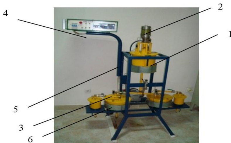
15-rasm. 1-aralashtirgich-tindirgich, 2-dvigatel; 3-idish; 4- datchik; 5-stoyka; 6-spiral.
