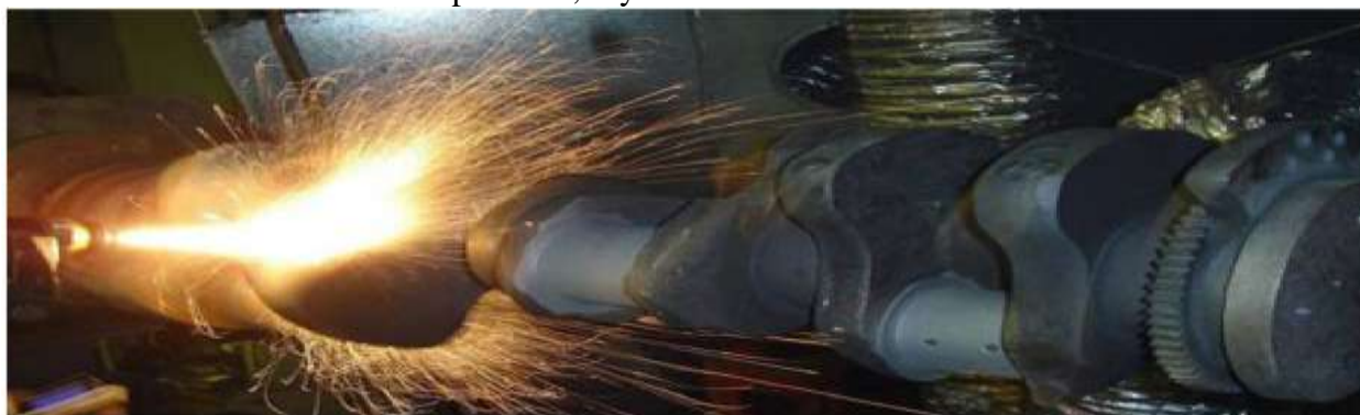
Rasim.2 Yuqori chastotali purkash apparatining kallagi . 1-detel sirti; 2—razmetal oqim; 3 — tokkondensatori; 4-suv bilan savitiladigan indiktor; 5-xavo kanali; 6-sim; 7 surish mexanizimning poliklari; 8-yunaltirivchi futulka.
