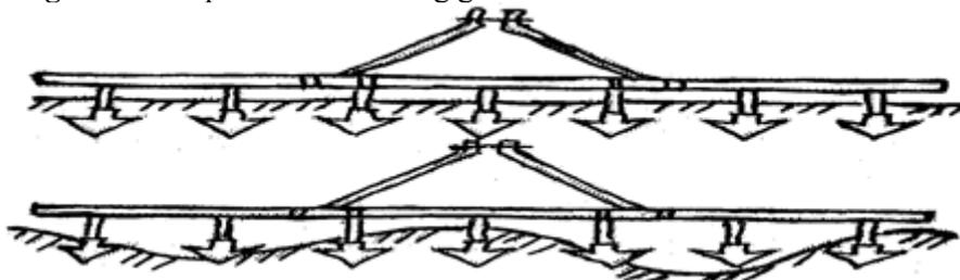
**Figure 2.** The process of working with a chisel-softener on levelled and uneven surfaces
