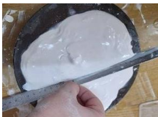
2-rasm. Gips xamirining normal quyugligini aniqlash.
