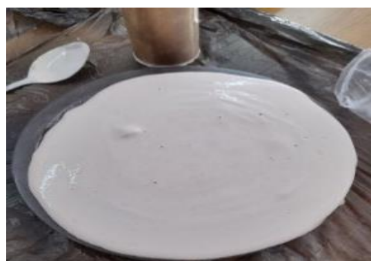
2-rasm. Gips xamirining normal quyugligini aniqlash.
