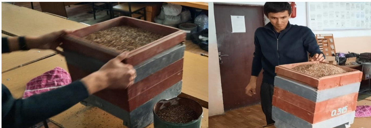
Figure 1. Determination of the granularity of multitasking vermiculite
