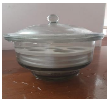
1-rasm. Suv shimuvchanligini aniqlash.
