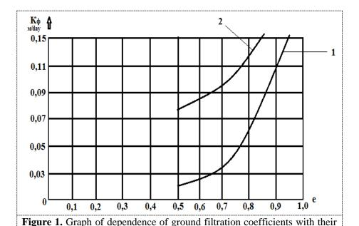
From the graph above, it is fair noting that even though the soil pore coefficients are the same, their active porosity is relatively high for the relatively large number of sand particles in light hydrocarbons, hence the increase in their permeability. Soil permeability is the property of the soil to transmit water and air and is one of the most important qualities [10].
