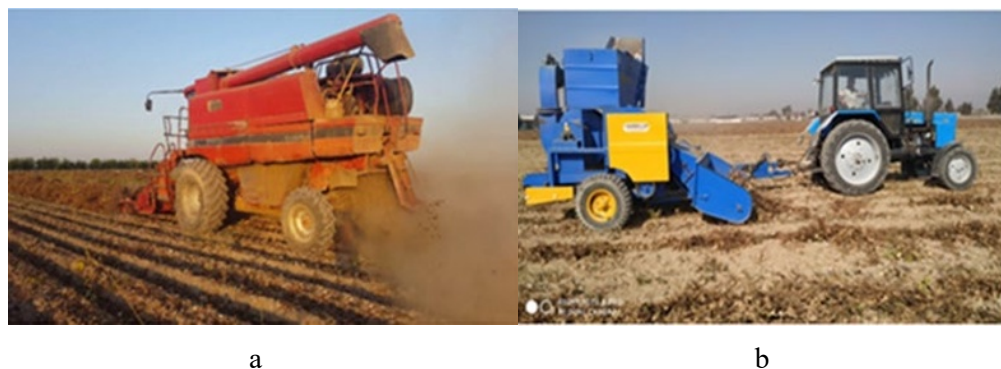
Fig. 2. The current technological process of mung bean harvesting: a – harvesting using a Keys-2166 grain harvester; b – harvesting using “Demireller” grinding machine made in Turkey.
