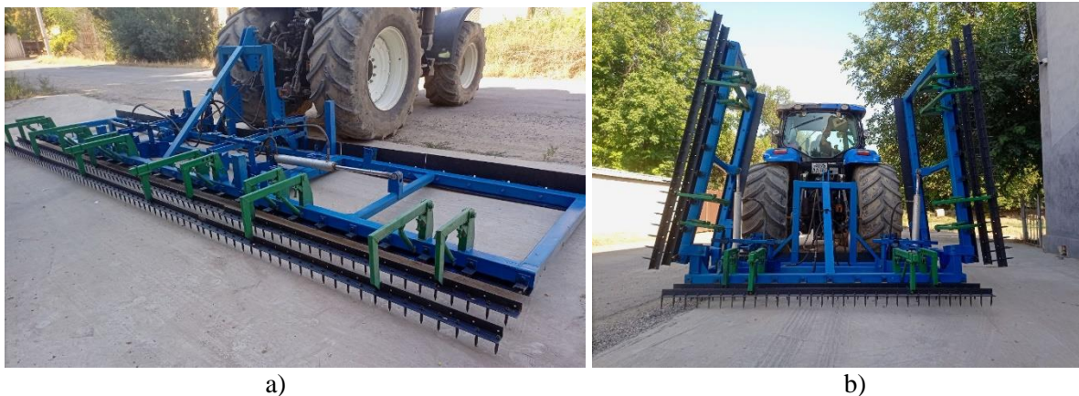
Figure 2. General views of the leveler in operation (a) and transport (b).
