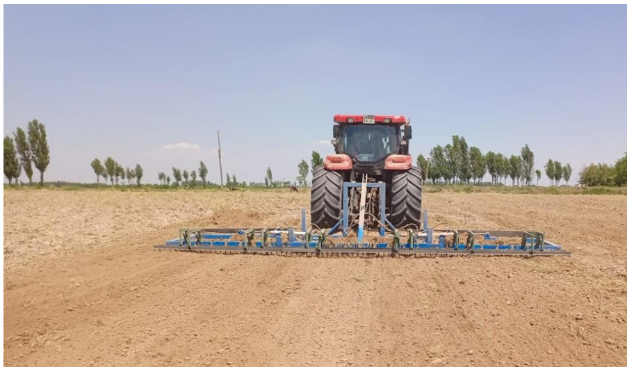
Figure 3. A view of the leveler in operation
