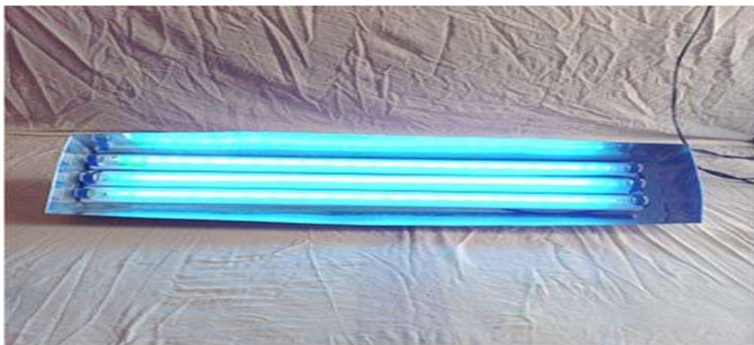
1-rasm. Gul urug'larini ultrabinafsha nurlantiruvchilaboratoriya stendi
