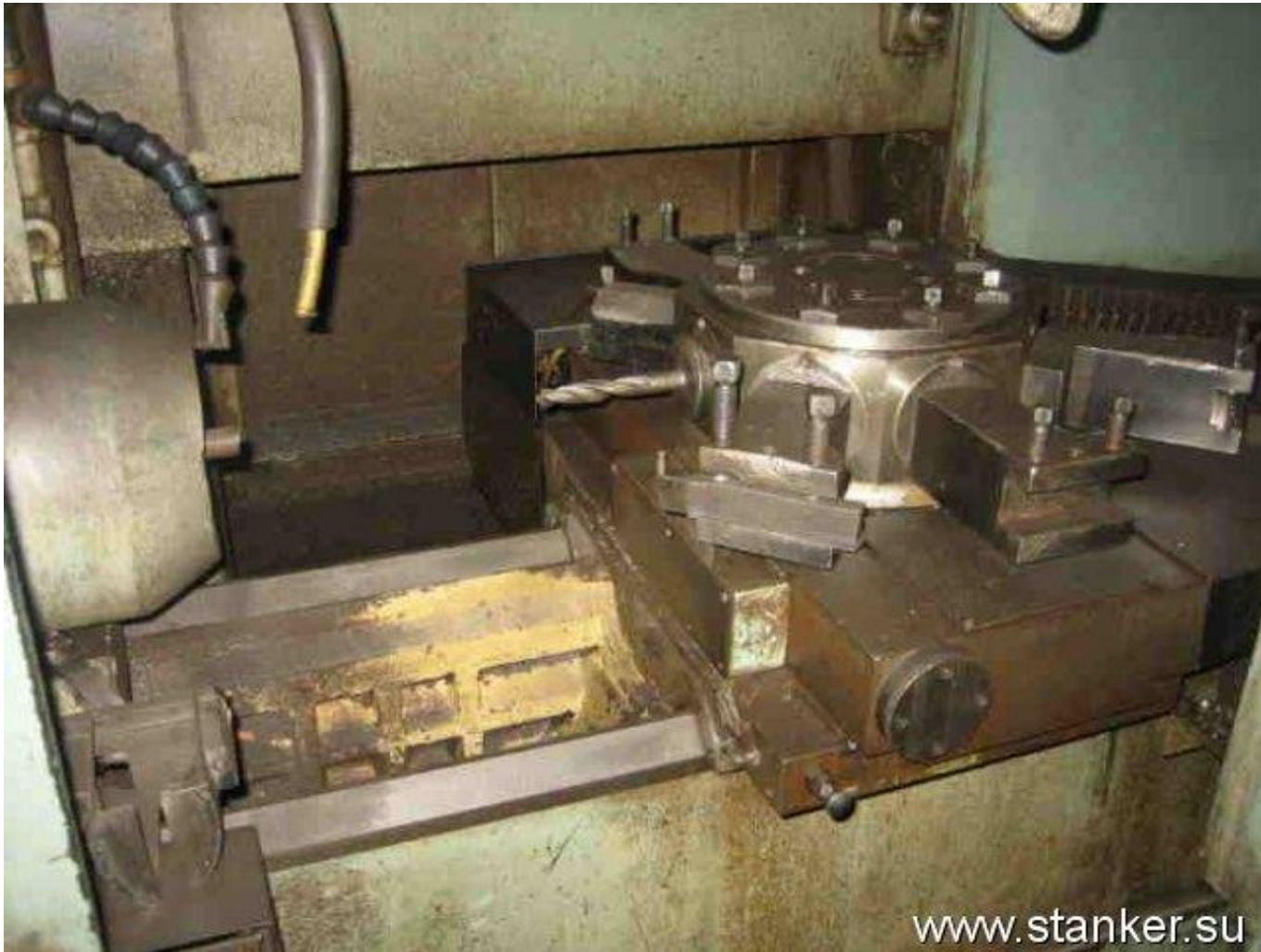
Tokar-revolver dastgohi (revolver kallagi vertikal o'q atrofida aylanadi)
