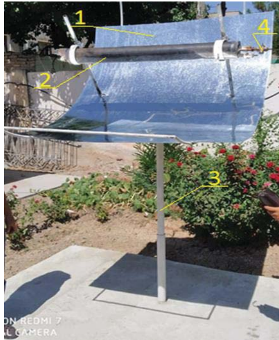
FIGURE 3. Heliopyrolysis unit with rotary reactor and solar concentrator: 1-parabolacylindrical concentrator; 2-reactor; 3-base foundations; 4-gas outlet
