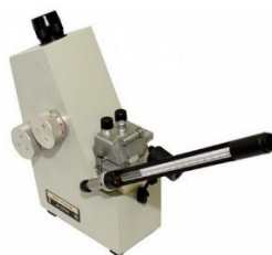
Eritmaning haroratini refraktometr IRF 454B2M" o'lchash " asbobi
