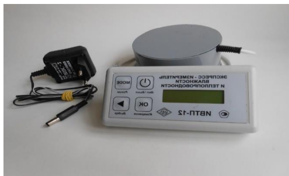
4.11 - rasm. Dilkometrik usulida namlikni o'lchash asbobi
