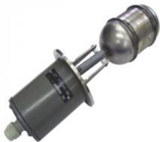
3.3-rasm. Tor diapazonda sathni o'lchash o'lchagichi: 1 – qalqovuch; 2-shtanga; 3- ko'rsatuvchi o'q; 4-idish
