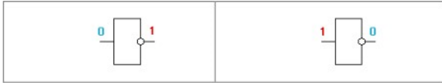
3.13-rasm. Inverterning ishlash prinsipi
