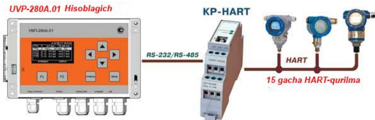
4.18-rasm. KP-HART kontrollerini tijorat hisobi tizimidagi UVP 280 liniya hisoblagichiga ulash sxemasi
