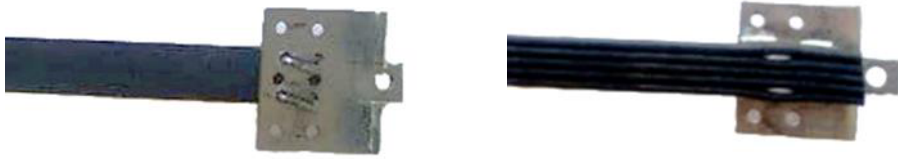
Fig. 4. Fastening of metal hooks to the poly-V-belt.
