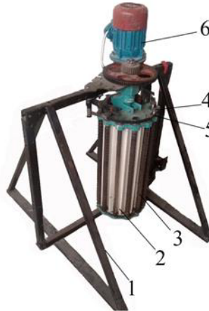
Fig 2. General view of the laboratory stand: 1 is frame; 2 is spindle drum; 3 is spindle; 4 is prototype roller; 5 is poly-V belt; 6 is electric motor.
