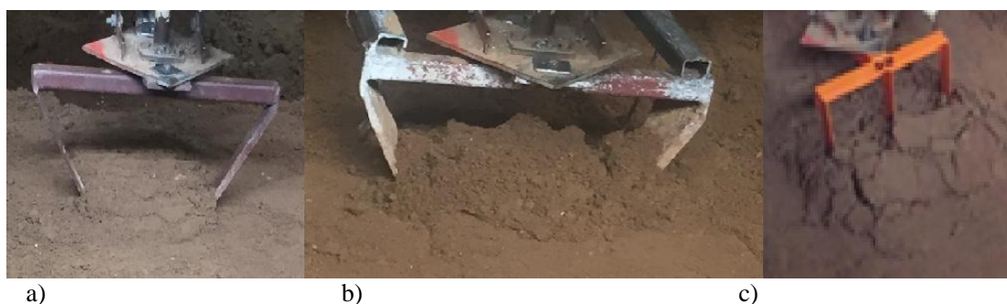
Figure 2. Loosening by passive working bodies of different types: a) V-shaped; b) volumetric deep loader; c) three-post
