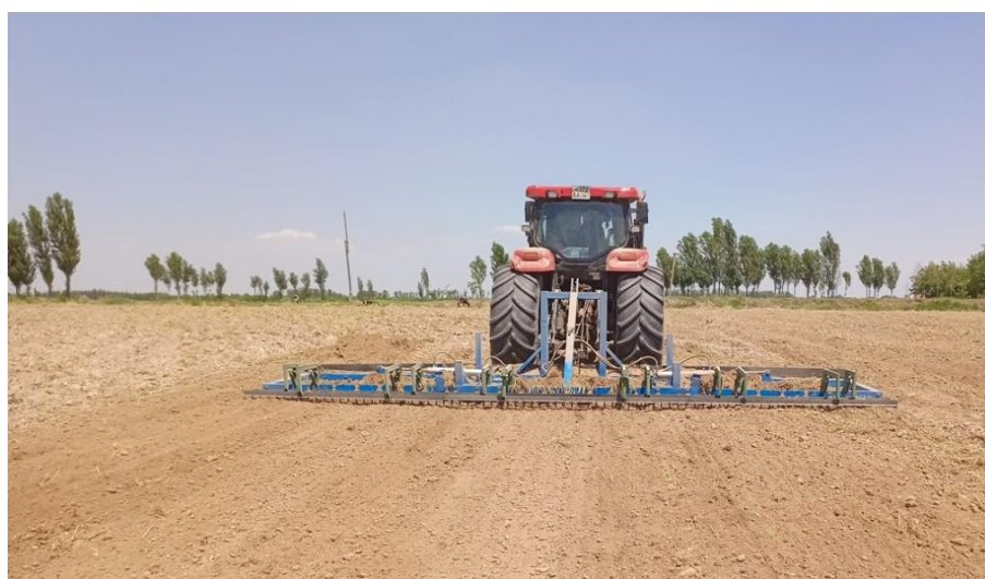
Figure 3. A view of the leveler in operation
