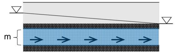
ie, homogeneous, isotropic aquifer with constant depth m:
