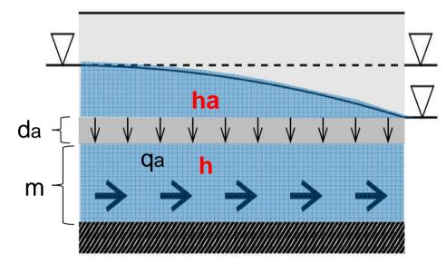
$$\frac{S}{T}\frac{\partial h}{\partial t} - \frac{\partial^2 h}{\partial x^2} - \frac{\partial^2 h}{\partial y^2} - \frac{h_a - h}{\lambda_a^2} - \frac{h_b - h}{\lambda_b^2} = 0 \qquad \lambda_a = \sqrt{\frac{Td_a}{k_{f,a}}}$$
