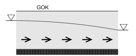
$$k_f \frac{\partial^2 h^2}{\partial x^2} = -2N, \quad q = -k_f \frac{\partial h}{\partial x}$$
