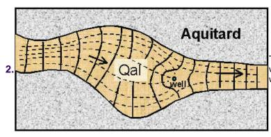
The effect of a producing well in a narrow, variable width, aquifer.
