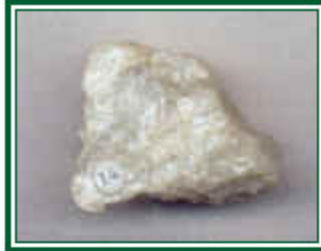
Talc talcum powder, paints, ceramics, paper coatings softest mineral (#1 on Moh's scale)
