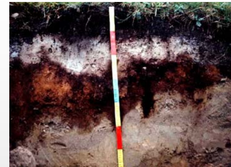
Normal Podzol from Ireland with a pronounced white eluvial horizon and separate illuvial humus and iron B horizons below ( Haplic Podzol )
