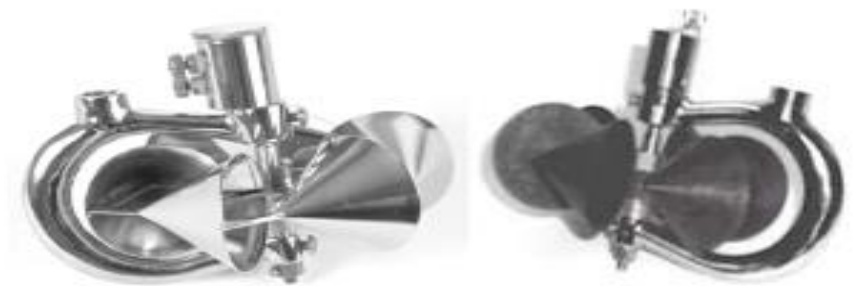
Рис. 10. Вертушка Прайса USGS TYPE AA-ICE MODEL 6240, USGS TYPE AA-ICE-P MODEL 6245 (Rickly Hydrological Company, США) (по [12; 19])
