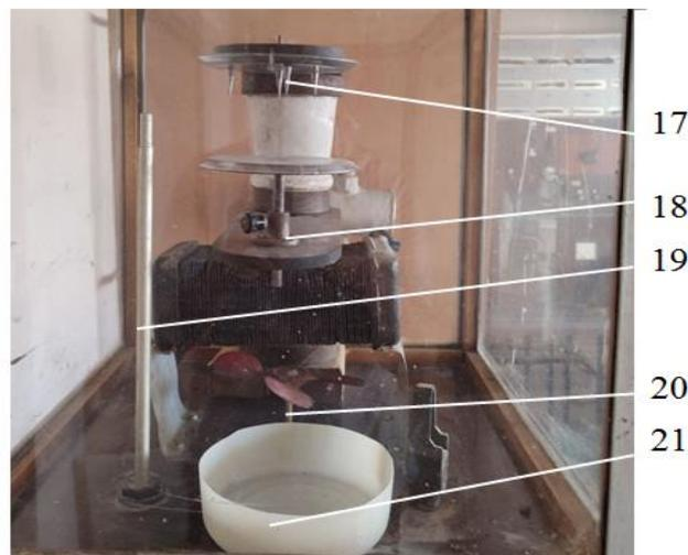
17 – needle electrodes; 18 – clamp for regulating the interelectrode distance; 19 – thermal resistance for M-1006; 20 – fan; 21 – tray for saturated saline solution
