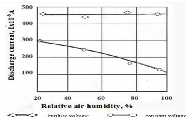
**Fig. 5.** Dependence of the discharge current on the relative humidity of the air and the effective voltage value of 35 kV (electric field strength 467 kV/m)
