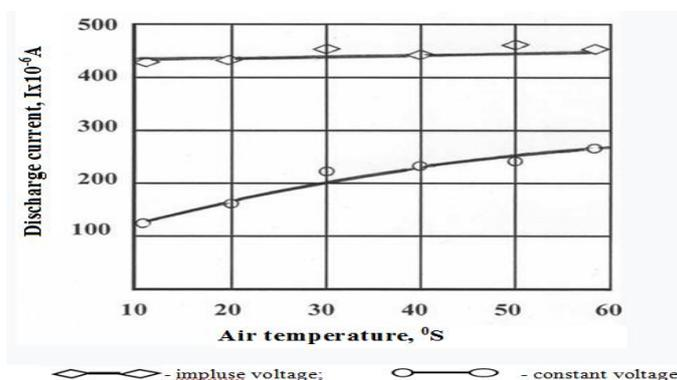
**Fig.4.** Dependence of the discharge current on air temperature at a relative humidity of 75% and an effective voltage value of 35 kV (electric field strength 467 kV/m)
