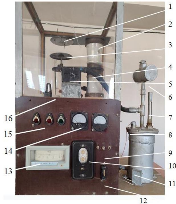
1 – potential electrode; 2 – support insulator; 3 – grounded electrode; 4 – pipeline; 5 – radiator;
