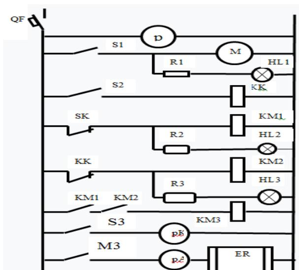
**Fig.1.** Schematic diagram of a climatic chamber for studying the influence of temperature and air humidity on corona discharge processes
