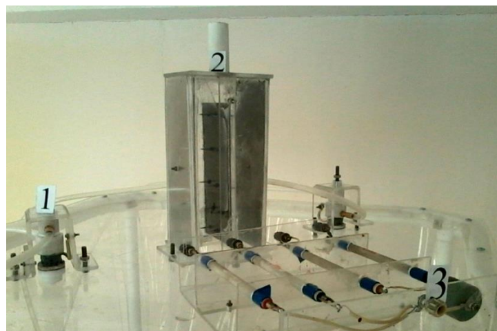
Figure 6. Equipment installed on the cover of the contact chamber: 1-pneumoelectrostatic atomizer; 2-aerosol separator; 3 - block of rectifiers
