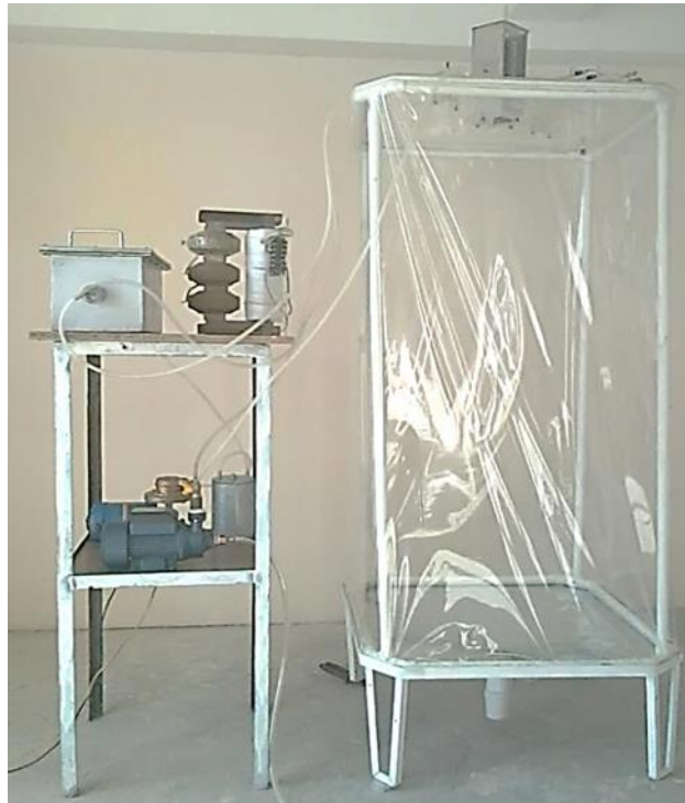
Figure 5. General view of the experimental setup for flow-through water treatment with ozone
