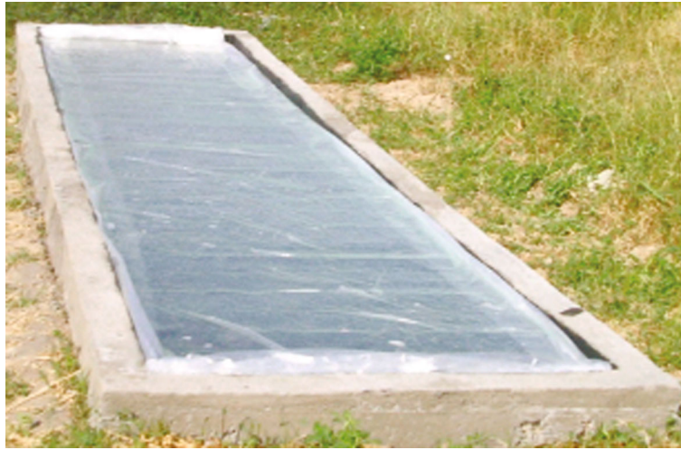
Fig. 1. Flat plate solar water heating collector (SWHC) with a surface area of 5 \text{ m}^2 with translucent coating.
